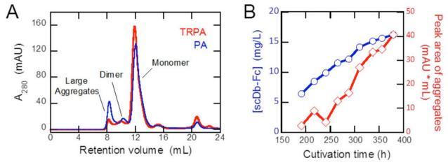
Figure 1 (A) Size-exclusion chromatography showing the elution profiles of Ex3-scDb-Fc purified with TRPA (red) and PA (blue). (B) Time-dependent formation of aggregates in CHO cell culture.
