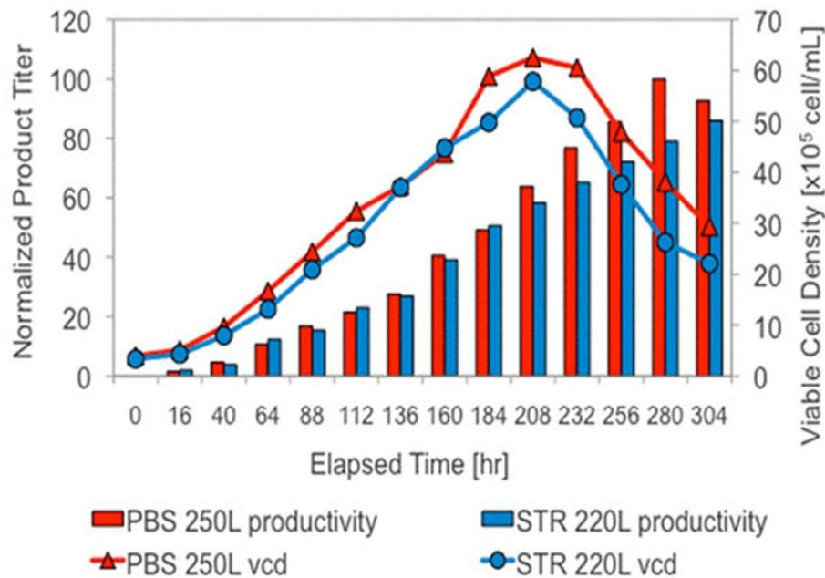
**Figure 1** Viable cell density and product titer comparison between 250L PBS bioreactor and 220L stainless steel bioreactor for an Fc-fusion protein
