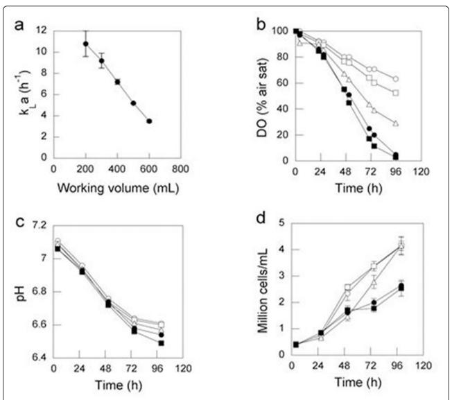
Figure 1 Effects of the  $k_L a$  on CHO-IgG cell cultures. The  $k_L a$  was measured in 1-L OSR with working volumes from 200 to 600 mL (a). The CHO-IgG cells were cultivated in 1-L OSR in 200 (b), 300 (c), 400 (d), 500 (e) and 600 mL (e). The DO (b), pH (c) and viable cell density (d) were measured at the times indicated. The shaking diameter was 5 cm.
