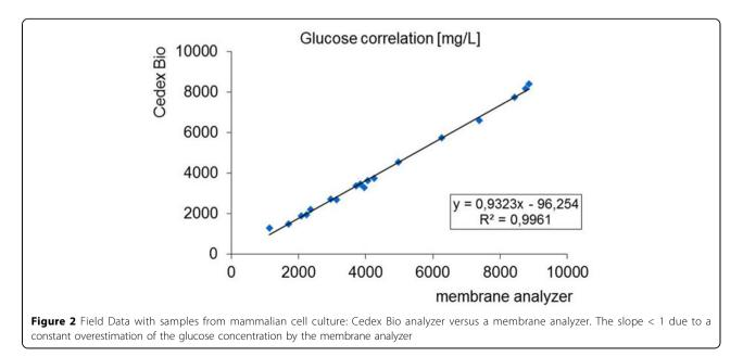
the Cedex Bio analyzer easily replaces the membrane analyzer with comparable batch data (Figure 2).
