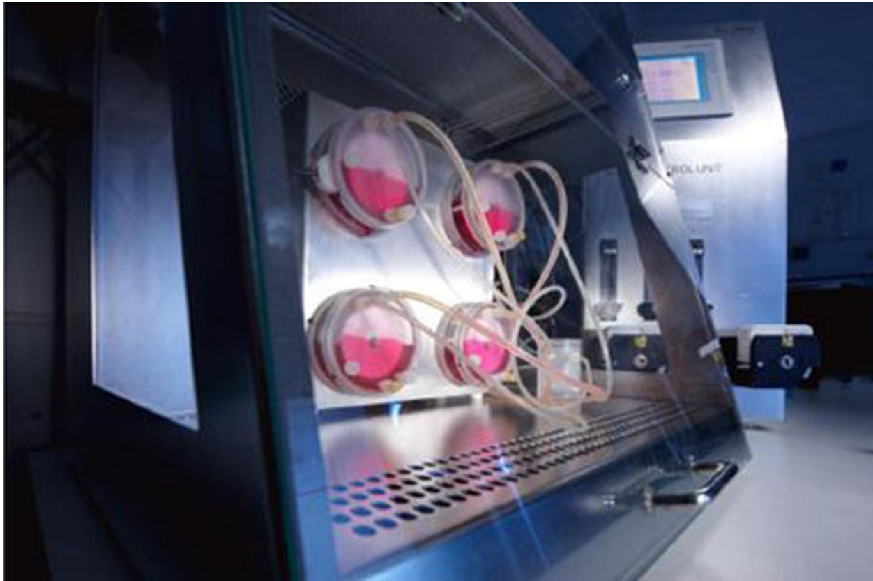
Figure 1 ZRP® bioreactor system (Zellwerk GmbH) with the special setup for performing four parallel cultivations.
