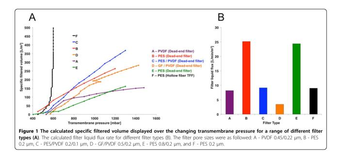
reduce the cost of the filtration. The PES hollow fiber TFF filter was able to filter over three times the sterile medium volume in comparison to the dead-end filters. The TFF filters displayed a similar range of filter liquid flux rates in comparison to the different filters types. This study showed that a hollow fiber TFF coupled with the use of a bearingless centrifugal pump provides a low-cost technology for the rapid large-scale 0.2  $\mu$ m sterilization of mammalian cell culture medium.
