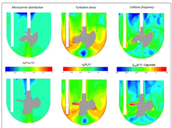
Figure 1 Microcarrier distribution (left), ratio of Kolmogorov scale to particle diameter (middle) and collision frequency for the elephant ear (top figures) and HTPG (bottom figures) impellers, operating respectively at  $N_{js} = 50$  and 85 rpm (P / V = 1 W m<sup>-3</sup>) and a Cytodex-1 concentration of 10 g L<sup>-1</sup>.
