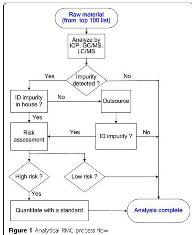
Figure 1 Analytical RMC process flow
