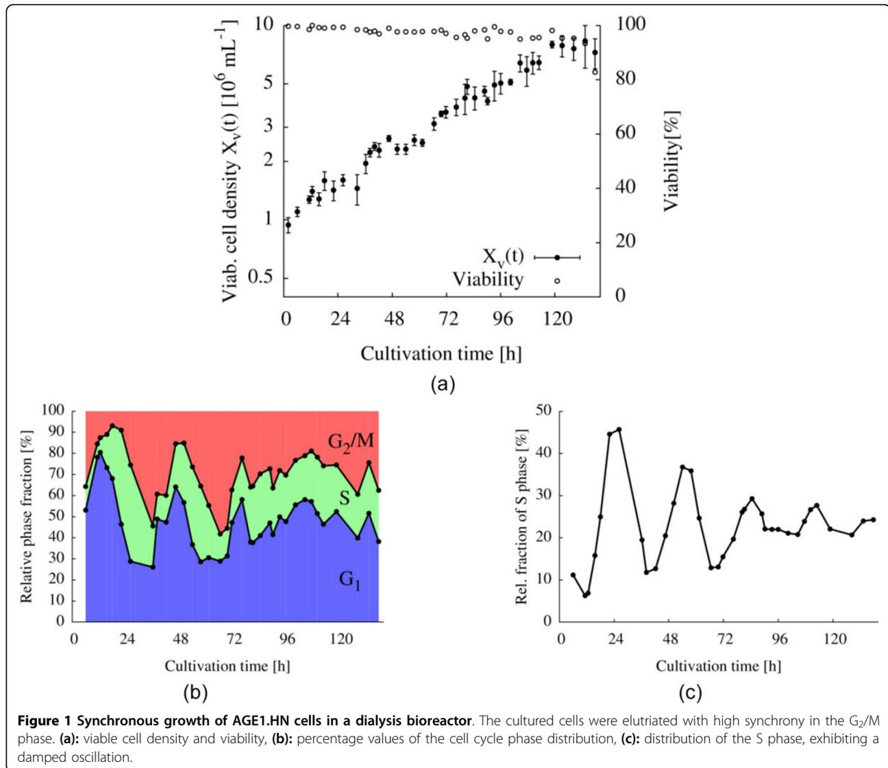
**Figure 1 Synchronous growth of AGE1.HN cells in a dialysis bioreactor.** The cultured cells were elutriated with high synchrony in the G<sub>2</sub>/M phase. **(a):** viable cell density and viability, **(b):** percentage values of the cell cycle phase distribution, **(c):** distribution of the S phase, exhibiting a damped oscillation.
