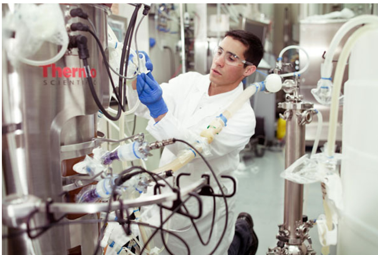
Figure 1 Hybrid intensified perfusion-based continuous bioproduction in a Thermo Scientific HyPerforma S.U.B. TK 250L supported by the Refine Technology ATF System.
