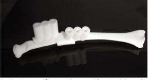
Patient specific cutting guide positioned on deformed radius both produced using additive manufacturing
