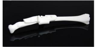
Patient specific drilling guide positioned on deformed radius both produced using additive manufacturing
