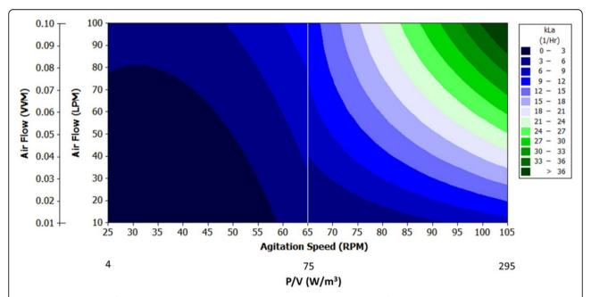
Figure 1 Contour plots for kLa<sub>02</sub>2080 values at various impeller agitation speeds and airflow rates. Two DOE models required to capture change in curvature with RPM (25 to 65 RPM & 65 to 105 RPM)
